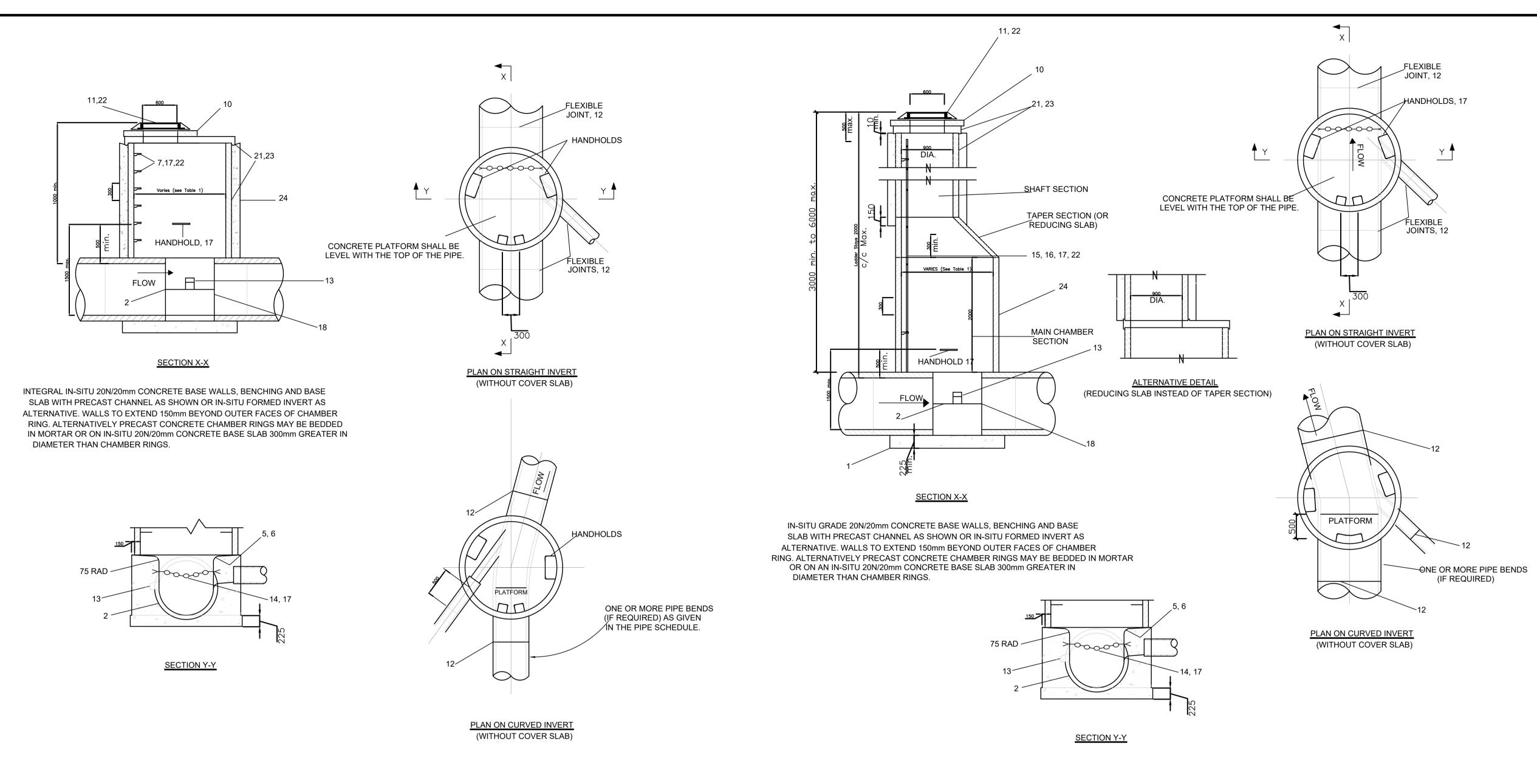
MANHOLE TYPE J (PRECAST CONCRETE MANHOLES)
